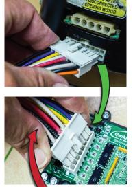
16-pin Connector from Motor to Qwik**Swap V3** Board
